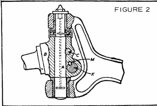
Figure 2 : axle assembly showing one type of king-pin arrangement
